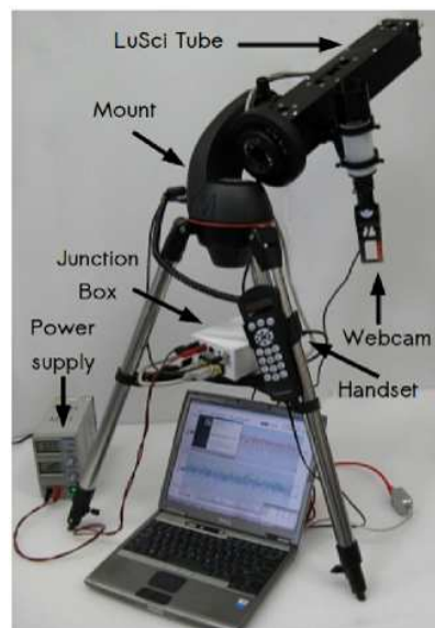
Figure 1. Portable ESO LuSci with the junction box containing a data acquisition module to store the data.
